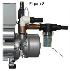
The inline strainer (Fig. 9) prevents debris from entering the solenoid and motor. If this strainer gets clogged, it could prevent water from entering the motor and potentially cause harm to the liquid ring vacuum. Inspect and clean this strainer quarterly. It can be cleaned by removing the internal screen with a 10mm open- end wrench. Rinse the strainer with tap water to remove any debris. Re-thread the strainer back into the hole it was removed from.
